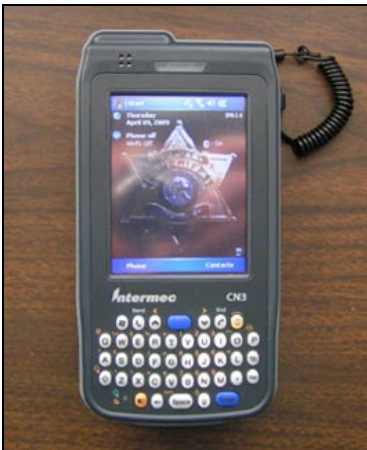
Ruggedized Intermec CN3 with Keypad, WAN Radio, and 2D Bar Code Scanner; Intermec headquarters are located in Everett, Washington.
